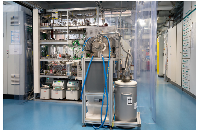
LPCVD equipment for deposition of wear protecting and functional coatings.
